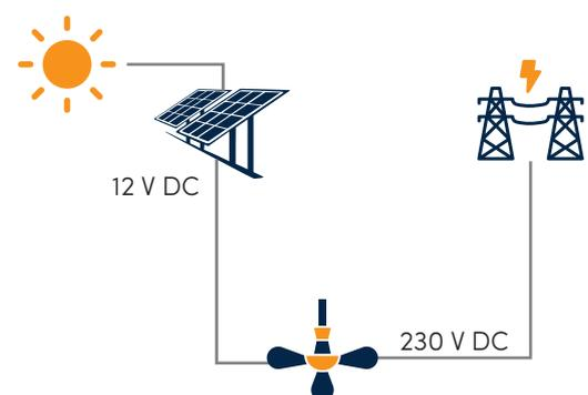
**b. Air conditioners (Videocon and Solar AirWorld):** These hybrid air conditioners runs on both AC and DC power with an intelligent power management technology that prioritises solar during daylight hours. The Solar AirWorld Hybrid AC product can also accept DC power directly from PV modules, without needing an inverter, controller, or batteries.
